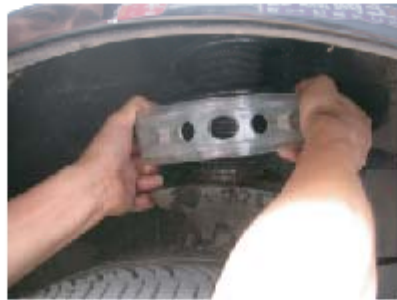
5. Also spray on the groove of Buffer and then install. It'd better put in the middle of the absorber.
