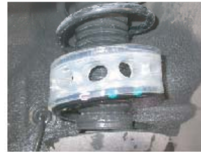
6. Check whether spring is fitted well in the groove. Then lift car down. Installation complete.
