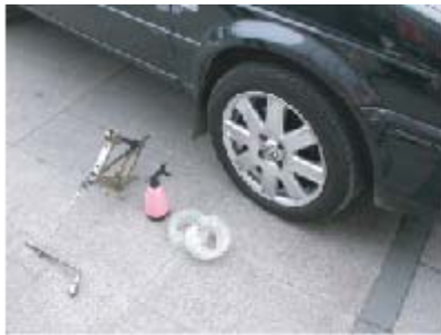
1. Prepare Buffer, jack, and soap water (In case of Urethane Buffer, grease and oil can be used)
