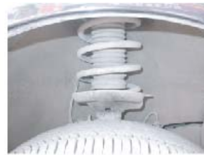
3. Then you can see that the spring is loosening.
